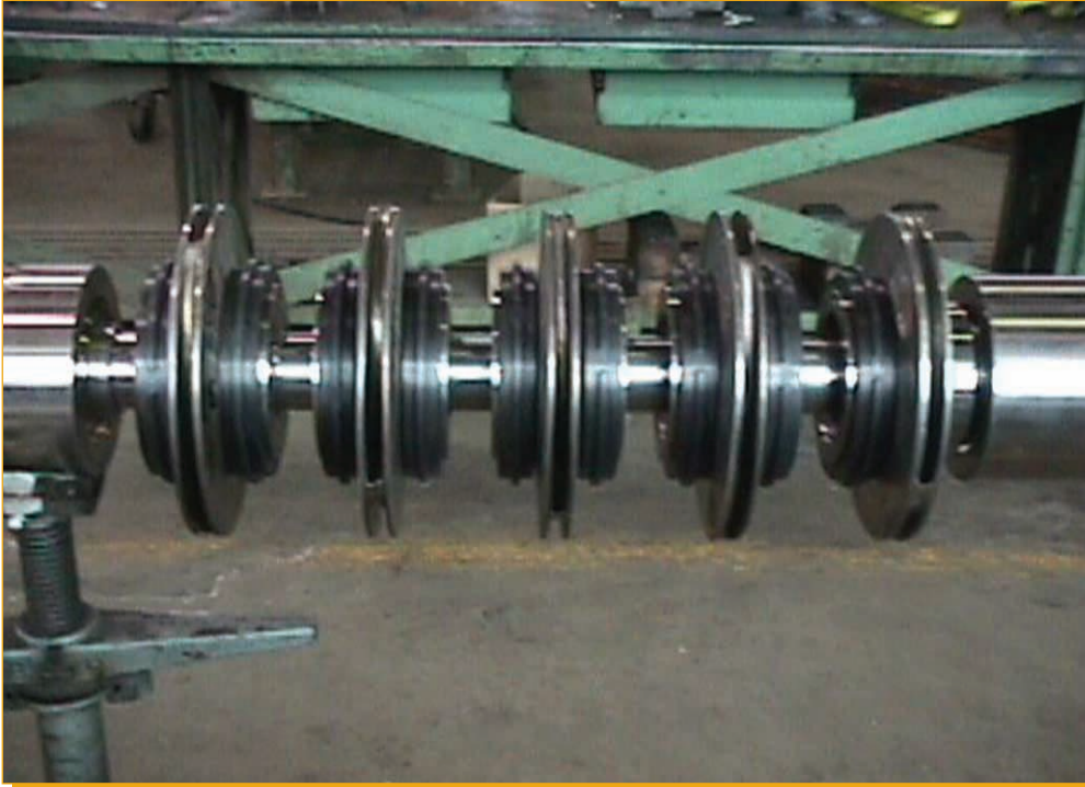
Figure 3. A large vertical turbine pump.
